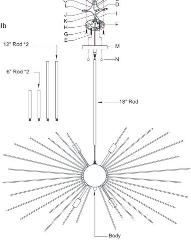
**Note:** Hanging rods of multiple lengths are provided to allow adjustment of the lighting fixture's suspension length.
