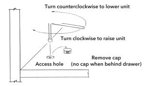
After alignment, replace the plastic cap.
